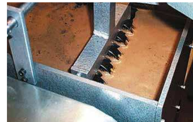
The various seal designs show a different level of performance in the contaminated environment of application.
